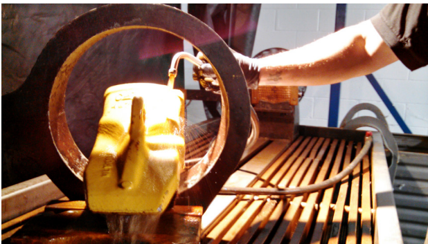
Wet fluorescent MPI is more reliable and more sensitive to very fine defects and more convenient than visible dry MPI.
