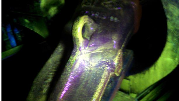
Wet fluorescent MPI is more reliable and more sensitive to very fine defects and more convenient than visible dry MPI.
