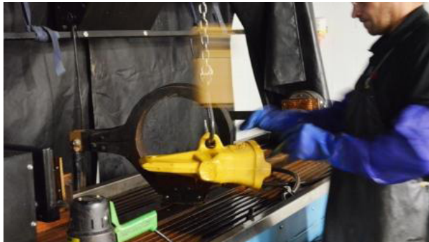
SCSI's wet horizontal MPI machine at our Peoria-Broadway facility, can accommodate parts up to 200 pounds.
