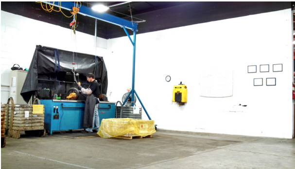
SCSI's wet horizontal MPI machine at our Peoria-Broadway facility, can accommodate parts up to 200 pounds.
